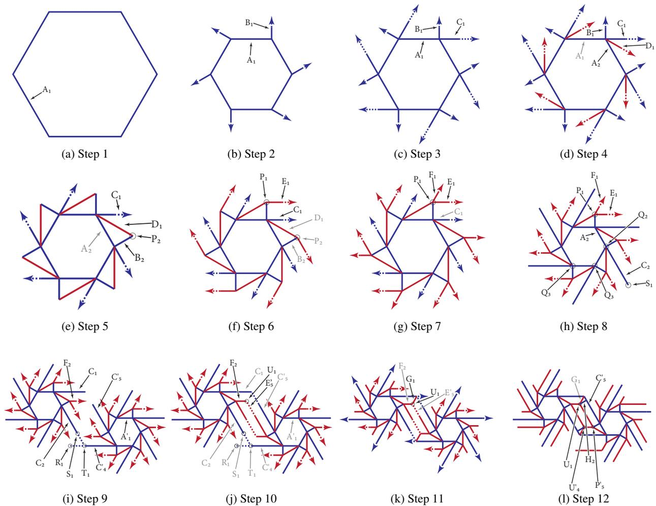
Figure 4: Step-by-step partial reconstructions of Huffman's "Three Axis Woven Design".
