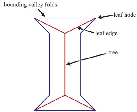
Figure 7: The components of a repeating unit.
